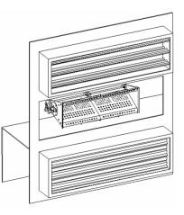
If the pressure drop is too high, in fresh mode only, remove or adjust the bypass damper blank-off panels, which will decrease the pressure drop. The return air damper opening may need to be adjusted to maintain the correct air flow pressure drop when switching back to return air mode.
