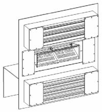
If the pressure drop is too high, in fresh and return air mode, remove or adjust the bypass fresh air and return air damper blank-off panels, which will decrease the pressure drop. If the correct air flow pressure drop is still not achieved adjust the blower drives to decrease the blowers RPM.
