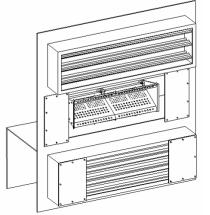
If the pressure drop is too high, in return air mode only, remove or adjust the return air damper and burner profile opening blank-off panels, and add the blank-off panels to the bypass damper, which will decrease the pressure drop.
